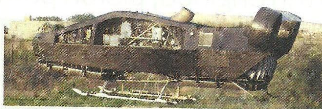
AirMule completed tethered tests in wind speeds of up to 50kt
